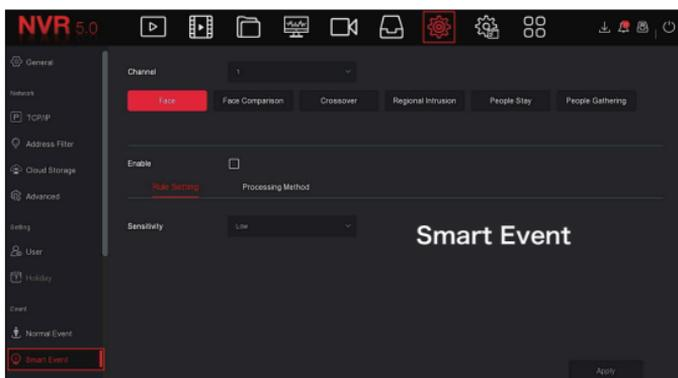
Step 2: Select the smart event alarm mode for setting the channel.
